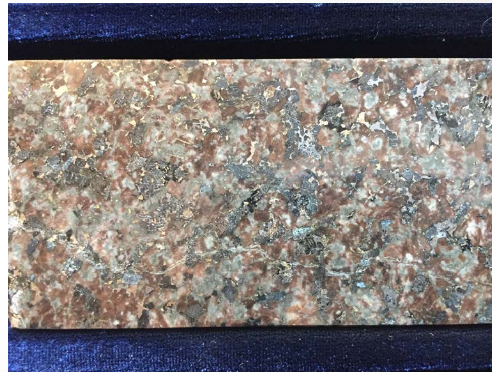
Gabbro-Gabbro-norite unit host to Campbell Zone. Photo of sample 35331 from ER09-19. 2.27 g/t TPM and 0.98% Cu+Ni
