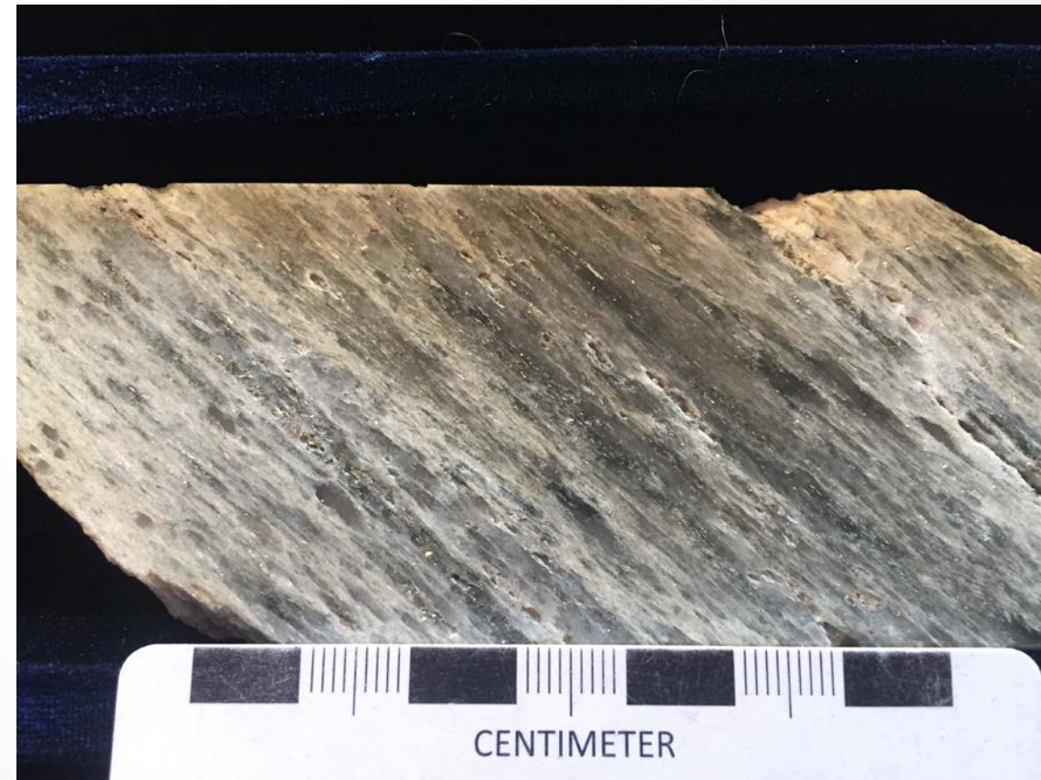
Sheared, altered felsic metavolcanics from Plomp Farm (NQ core) samples
