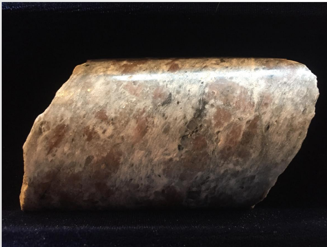
Sheared, altered felsic metavolcanic with andalusite porphyroblasts from Plomp Farm (NQ core)
