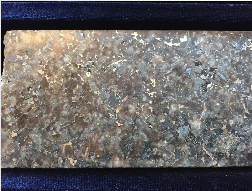
Gabbro-Gabbronorite unit host to Campbell Zone. Photo of sample 35330 from ER09-19. 2.33 g/t TPM and 0.95% Cu+Ni
